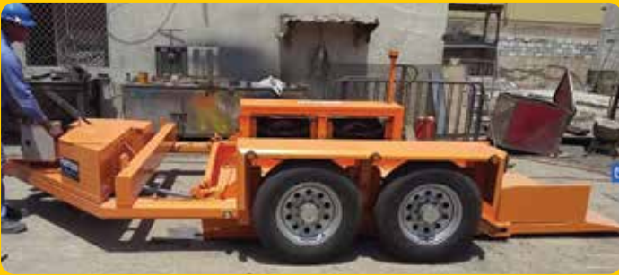
Lower entire deck to ground level
